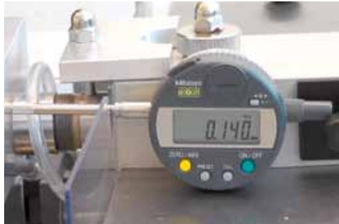
\mu -accurate sample positioning with digital micrometer
