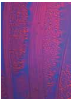
GFRP thin section Polarization microscope
