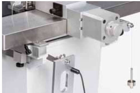
Parallel control system with precise feed control and automatic sample positioning
