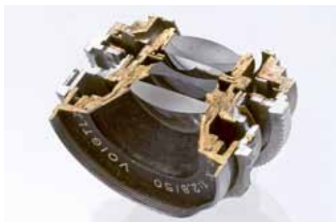
Cut of a camera lens
