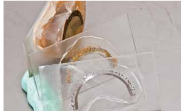
Processing thin sections – e.g. titanium acetabular cup
