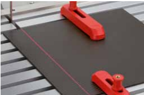
EXAKT 311 – Cutting of CFC sheet for tensile testing
