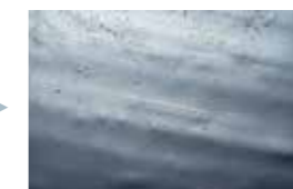
Crack of resin molded article (350x)
