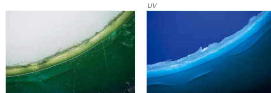
Scratches on circuit board (80x)
