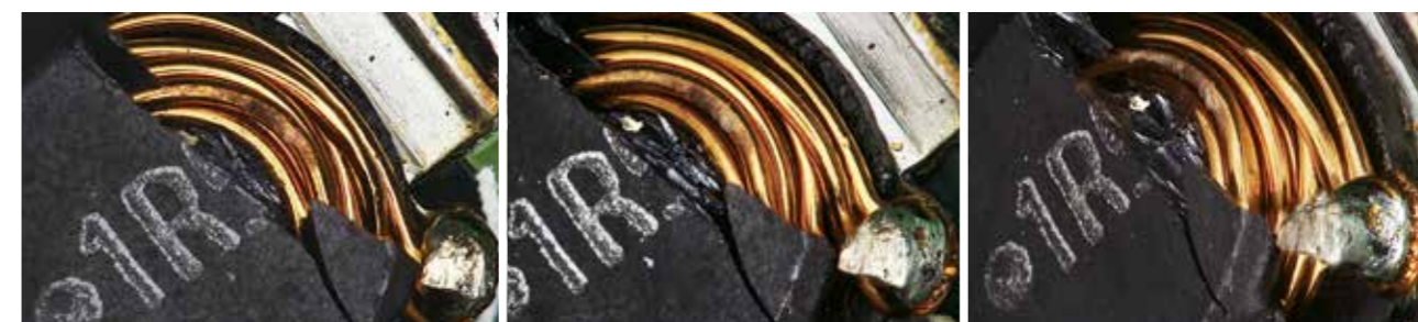
Crack of mounted component (60x, 0 degree)
