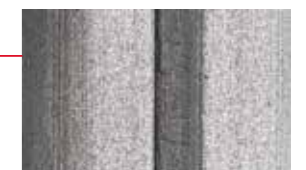
Junction on the inner wall of aluminum pipe (50x)
